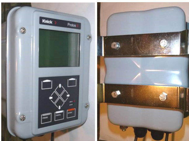
Picture 5 Protos II without visible damage or defects after the harmful gas test
