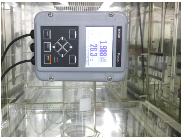
Picture 3 Protos II – operating with displayed values in the corrosion test chamber K 350 at the beginning of the harmful gas test
