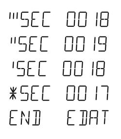
Electrode response time of last calibration Electrode response time of second last calibration Electrode response time of third last calibration Electrode response time of first calibration End of Electrode Data menu.
