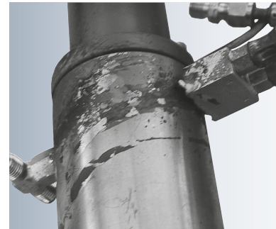
Conventional retractable fittings: Tangled hoses (left) and deposits on unprotected limit-position mechanism (right)
