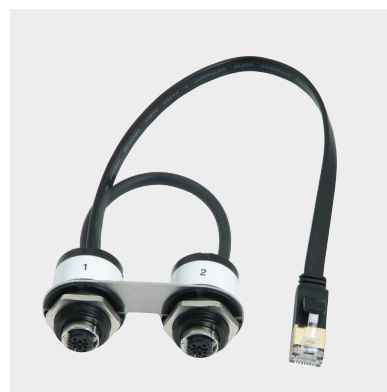
The Y cable connects an RJ45 socket on the Stratos Multi E461N to two D-coded M12 sockets and is used for PROFINET data transmission.
