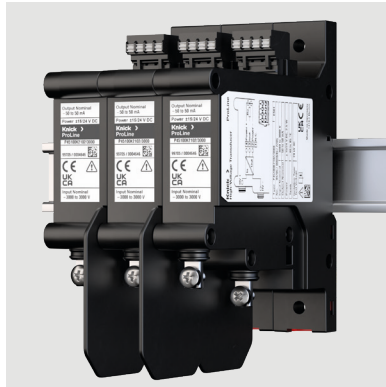
DIN rail mounting with ZU1471 partitions
