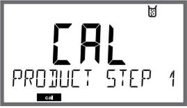
The display shows 'CAL' in large digits, with 'PRODUCT STEP 1' below it. There are navigation arrows on the left and right sides, and a small icon in the top right corner.  | Ready for calibration.<br>Hourglass blinks.<br>Select calibration method: P_CAL<br>Press <b>enter</b> to proceed. | Display (3 sec)<br>Now the device is in HOLD mode.                   |
