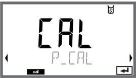
The display shows 'CAL' in large digits, with 'P_CAL' below it. There are navigation arrows on the left and right sides, and a small icon in the top right corner.            | Select product calibration.<br>Press <b>enter</b> to proceed.                                                     | If an invalid code is entered, the device returns to measuring mode. |
