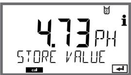
The display shows '4.73 pH' in large digits, with 'STORE VALUE' below it. There are navigation arrows on the left and right sides, and a small icon in the top right corner. | Take sample and save value.<br>Press <b>enter</b> to proceed.                                                     | Now the sample can be measured in the lab.                           |
