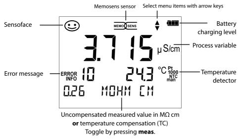
Press the **set** key to access configuration mode. Prior to measurement, a configuration should be performed to match the connected sensor and the desired measurement performance. Furthermore, you can select the suitable calibration method. The following table gives you an overview. Factory settings are shown in **bold print**.
