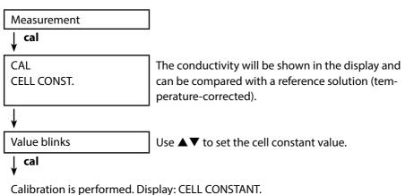
The meter then automatically returns to measuring mode.
