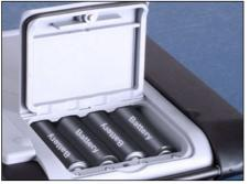
With four AA batteries, the Portavo has an operating time of over 1000 h. Open the battery compartment on the rear of the device. Be sure to observe the correct polarity when inserting the batteries (see markings in the battery chamber). Close the battery compartment cover and fasten it finger tight.
