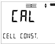
Calibration (Calibration by entry of cell constant)
