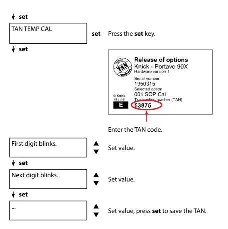
After correct input of the TAN, the device signals "PASS" – The option is now available.
