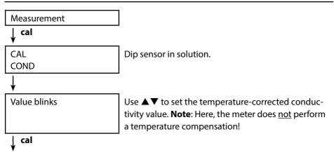
Calibration is performed. Display: CELL CONSTANT.
